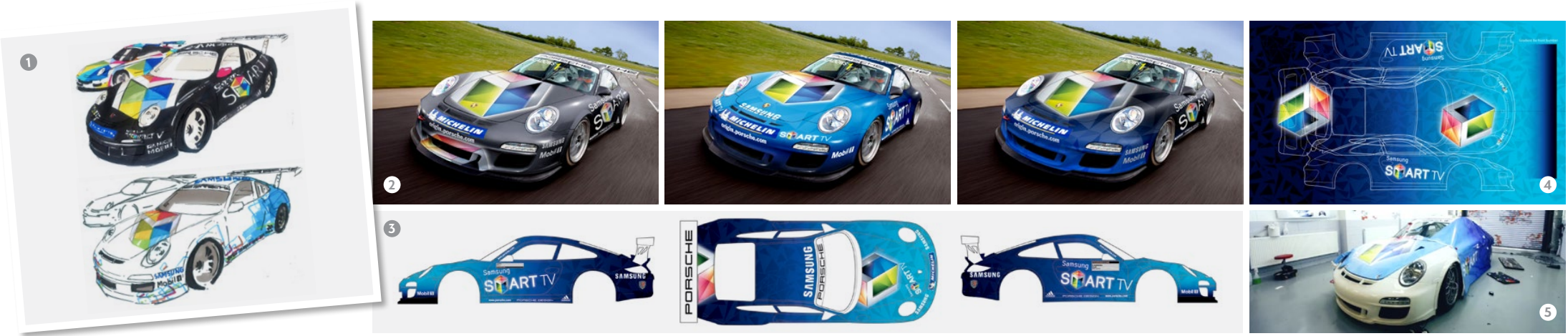
Above, car livery life cycle: 1 Concept illustrations from creative director. 2 Various Photoshop mockups for concept approval. 3 Final technical mockups for client approval. 4 Complete artwork supplied for large format digital vinyl printer. Special care taken with artwork preparation to ensure panel alignment on car due to the unique continuous, seamless wrap design. 5 Final vinyl artwork wrap application.
